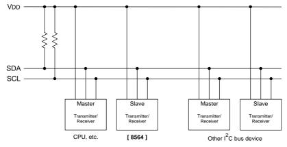
Any device that controls the data transmission and data reception is defined as a "Master".
